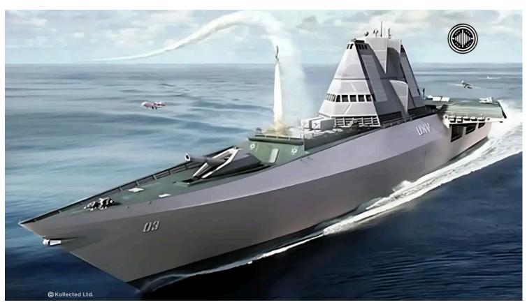
The UXV Combatant, a bold British concept warship unveiled in 2007, was designed to lead a new generation of drone-carrying vessels but never progressed beyond the design stage. Developed by BVT Surface Fleet, now BAE Systems Maritime, the proposal aimed to merge traditional firepower with cutting-edge unmanned operations across air, surface, and underwater domains.
