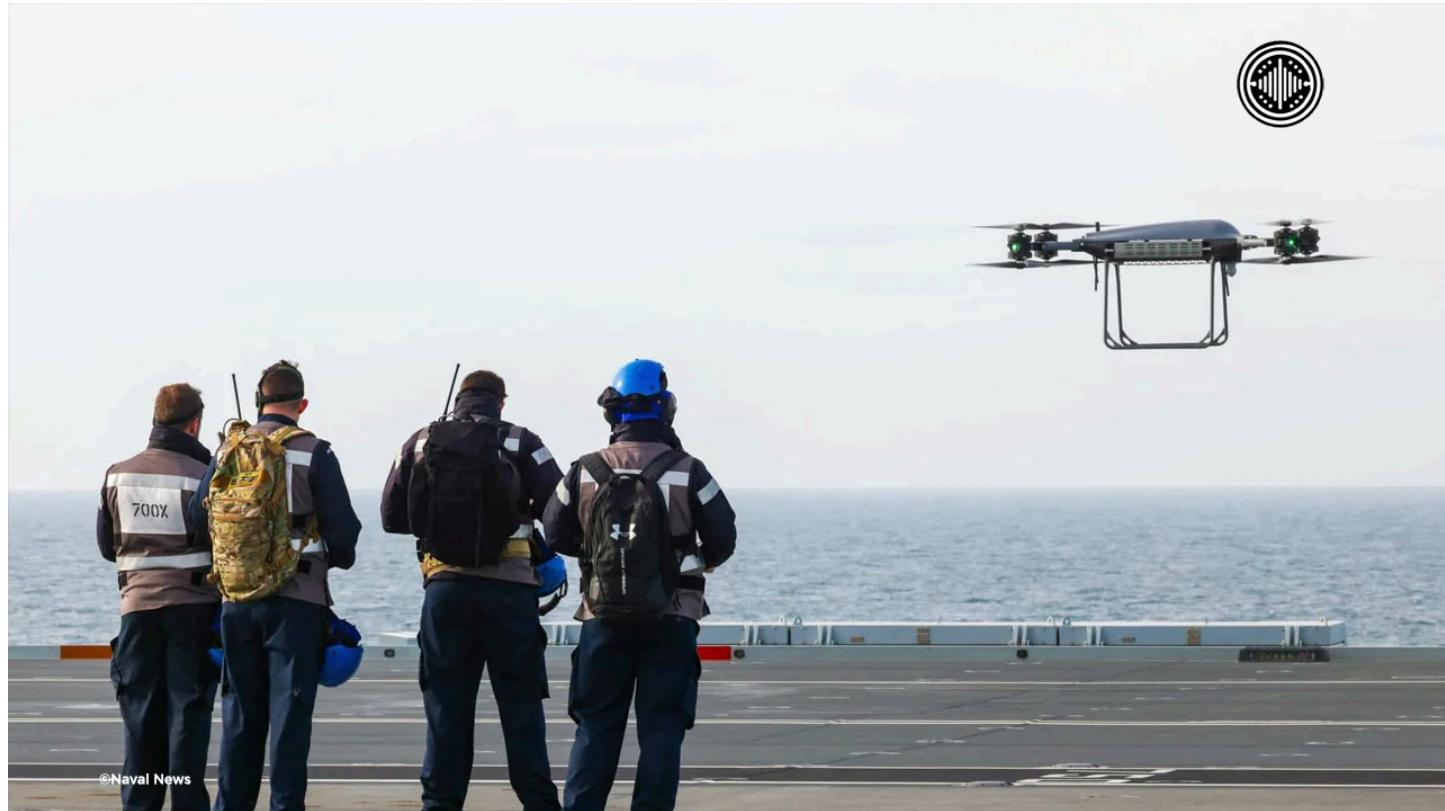
During Exercise Talisman Sabre 2025, the Royal Australian Navy (RAN) tested a drone-based delivery system designed to streamline logistics and reduce reliance on helicopters for supply transport. The trial took place off Shoalwater Bay, Queensland, and involved the Callisto 50 logistics drone delivering a six-kilogram repair part to HMAS Choules. The delivery was completed over a distance of 6.5 kilometres in just over eight minutes.
